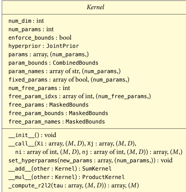
Figure E.4: Class diagram for the Kernel abstract class. __call__() is a placeholder method and must be implemented in any subclass which implements Kernel .
